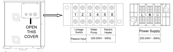
MARNING: The maximum power of external electric heater is 3 kW.
