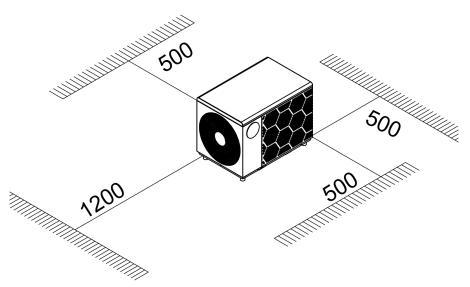
Do not put anything less than one meter in front of the heat pump.
