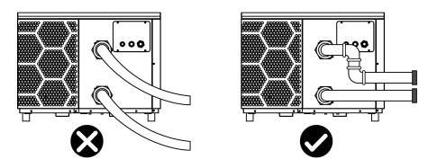
2. In order to guarantee the heating efficiency, the water pipe length should be  $\leq$ 10m between the spa/pool and the heat pump.
