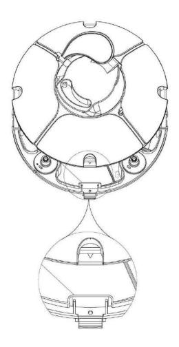
g. When charging, it is strictly forbidden to face the bottom up to prevent the swing plate from being crushed.
