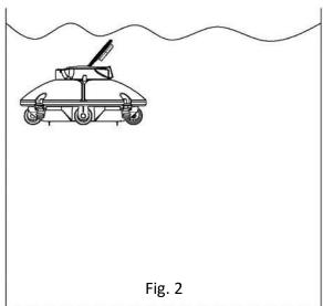
b. Put into or lift out of the pool with the cleaner bottom towards the wall to avoid any possible scratches to the pool.
