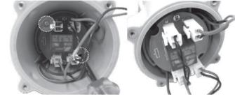
4. Detach all 4 cable connectors by pressing on the clip and detach it simultaneously. Remove the whole module out of the chamber to expose the battery. Remove the battery and wrap its connector end with insulating tape in order to avoid short circuit caused by the contact of both wire terminals. wire terminals.
