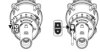
2. Connect the USB charging cable to the charging adaptor, then plug the charging adaptor into the power source. Once the electric vacuum begins to charge, the indicator light will turn red. Normally, it takes about **4.5 - 6** hours to reach a full charge. The indicator light will turn green once the electric vacuum is almost fully charged.
