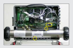
Place your new heater into the heater rack. Insert the
