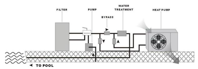
If your installation is equipped of a water treatment with product adductions (chlorine, brominates, salt...) the by-pass must be installed before the water treatment, with a non-return valve between the by-pass and water treatment.
