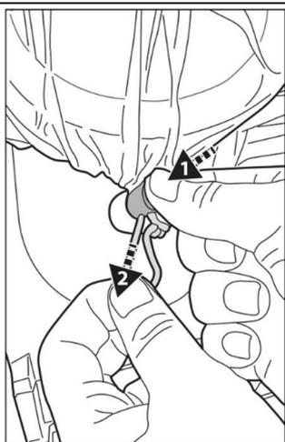
While holding the cord, press on the cord fastener and push it under the flange. TIPS: To secure the filter bag, when pushing the cord fastener under the flange, pull one cord instead of two cords as shown in diagram.
