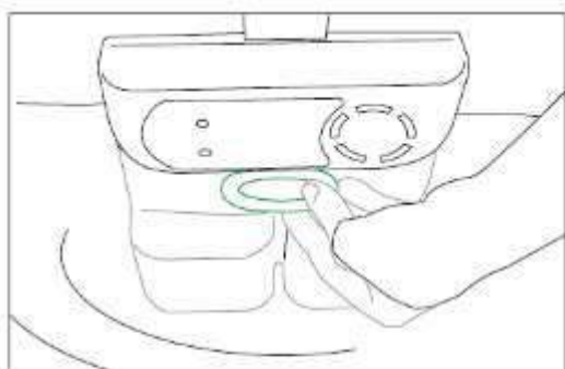
Remove the screw cover (if any) using a flat screwdriver.
