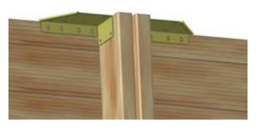
Figure 18 – Fastening metallic support brackets to the top of the supporting braces
