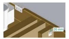
Figure 35 – Location of the lock striking plate
