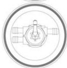
CIRCULATION: Water from the pump returns directly to the pool without passing through the filter.
