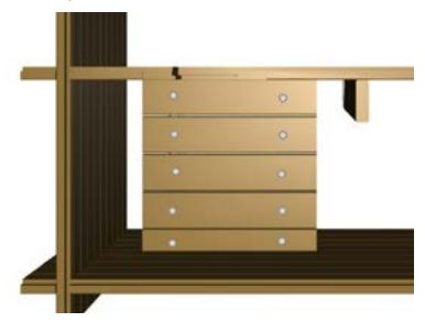
Figure 15 – Assembling the base of the plant housing portion of the box
