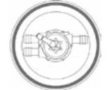
BACKWASH: Water from the pum crosses the filter from the bottom to the top and is then routed to waste taking with it dirt and debris trapped by the filter.
