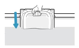
After placing the robot in the water, please wait 2-3 minutes for it to prepare for Tip cleaning. The robot will sink to the pool floor and release the air from the buoyancy chamber, then begin cleaning automatically.
