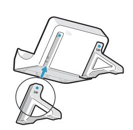
2 Install it onto the robot with the interface facing down
