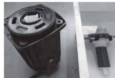
5. Put pump body in a vertical position and fill with a mild lime scale remover (like cleaning vinegar). Immerse rotor in a plastic bowl/container filled with the same lime scale product and leave both for 24 hours. After 24h rinse off with water and re-assemble pump.
