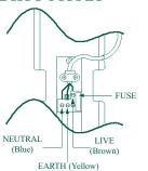
Mains electrical cable is not supplied with the unit. This unit must be connected to permanent wiring. A switch with 3mm contact separation must be provided in the fixed wiring to provide disconnection from the electricity supply.
