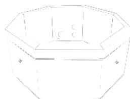
6) Adjust the 8 segments until they form a perfect round shape. Then, ensure that the holes for the outer liner connection and the holes in the foam wall are still aligned.
