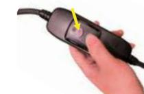
4. Press the «RESET» button, the indicator light turns red. The RCD works properly.
