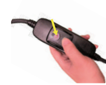
4. Press the «RESET» button, the indicator light turns red. The RCD works properly.
