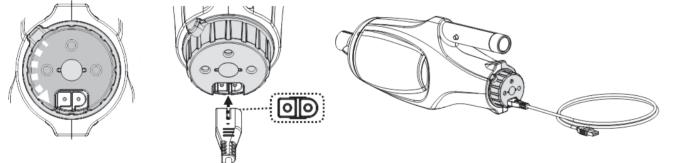
Connect the USB charging cable to the charging adaptor, then plug the charging adaptor to the power source.
