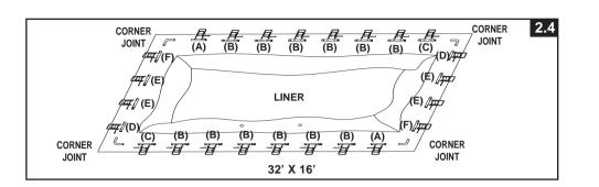
**3.** Be sure the liner is opened and spread out to its fullest extent on top of the ground cloth. Starting with one side, slide the "A" beams first into the sleeve openings located in each corner. Continue with "B" beam snapping into the "A" beam, and another "C" beam snapping into the "B" beam (see drawing 3).
