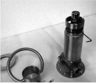
7. Loosen the socket-head screw on the aerator so that it can be detached from the progressive cartridge.
