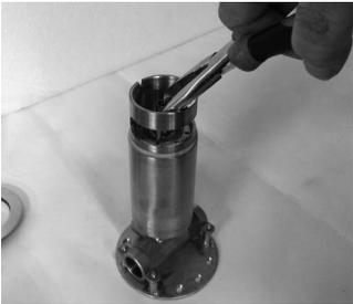
9. Using pliers, unscrew the inner ring from the cartridge.
