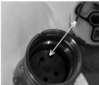
12.NB: There is only one correct way to reinsert the cartridge.
