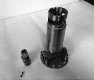
8. Remove the aerator from the casing.
