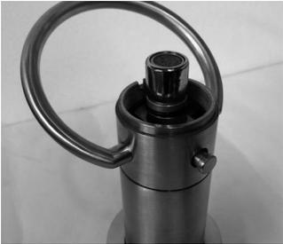
5. Take out the pin and remove the ring handle.
